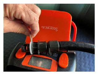
When using a SereneLife Air Pump, or pump with similar fitting, use the thinnest washer provided with the pump (slightly thicker than a USA quarter).
