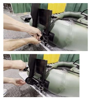
Insert Bungee chords from top-down, above motor mount cross bar and around rudder bracket.
