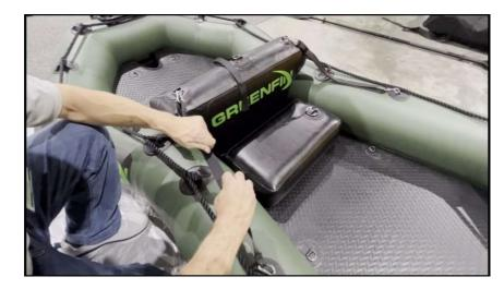
When operating your boat with a motor, best performance is achieved when the front seat and backrest are positioned near the middle portion of the air deck. Too far forward in the boat will make your boat front-heavy in waves.
