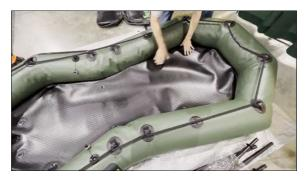
Inflate Main Tubes from 50% to 100% before tucking in deflated air deck.
