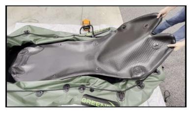
Reinflate Air Deck to its full shape for easy drying and cleaning.
