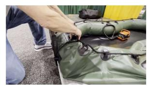
Insert Motor Mount when boat is ½ inflated. Do not attempt to insert motor mount in fully inflated boat.
